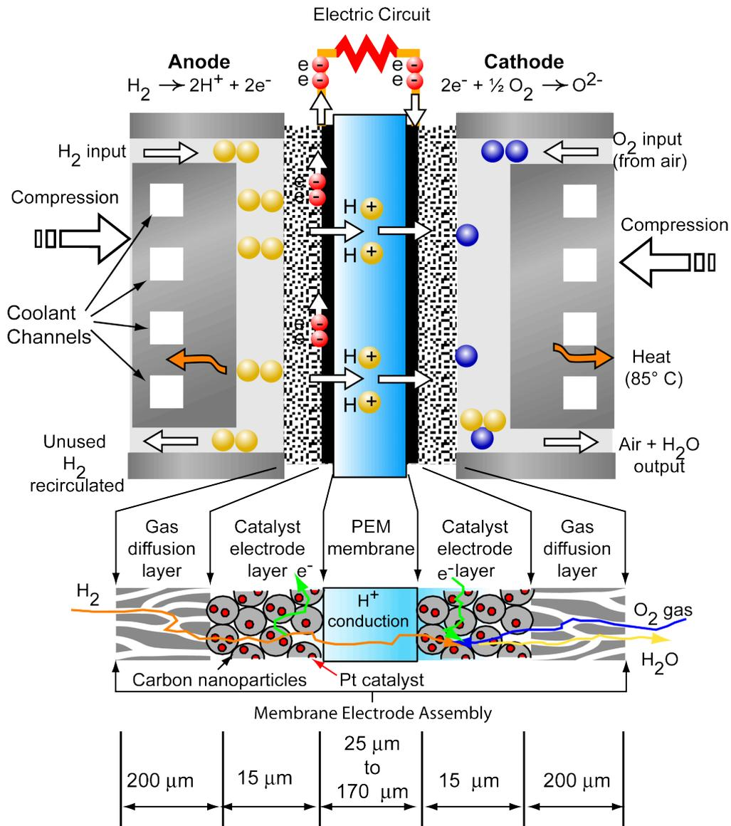
**Figure 2: Diagram of a PEM fuel cell.**
