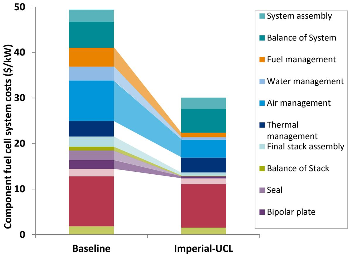
**Figure 20: How the Imperial/UCL fuel cell design reduces cost compared to current leading technology**
