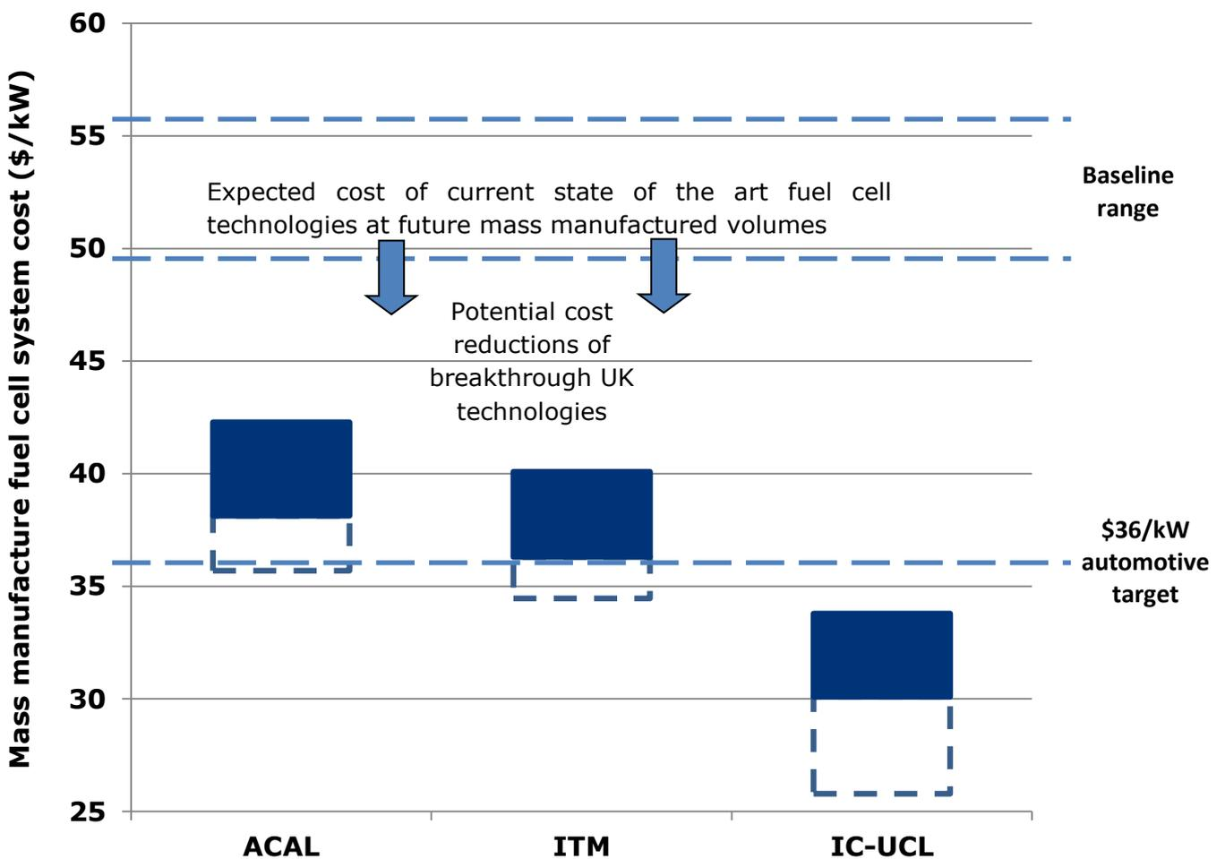
**Figure 8: Ranges of automotive fuel cell system costs at mass manufactured volume.**
