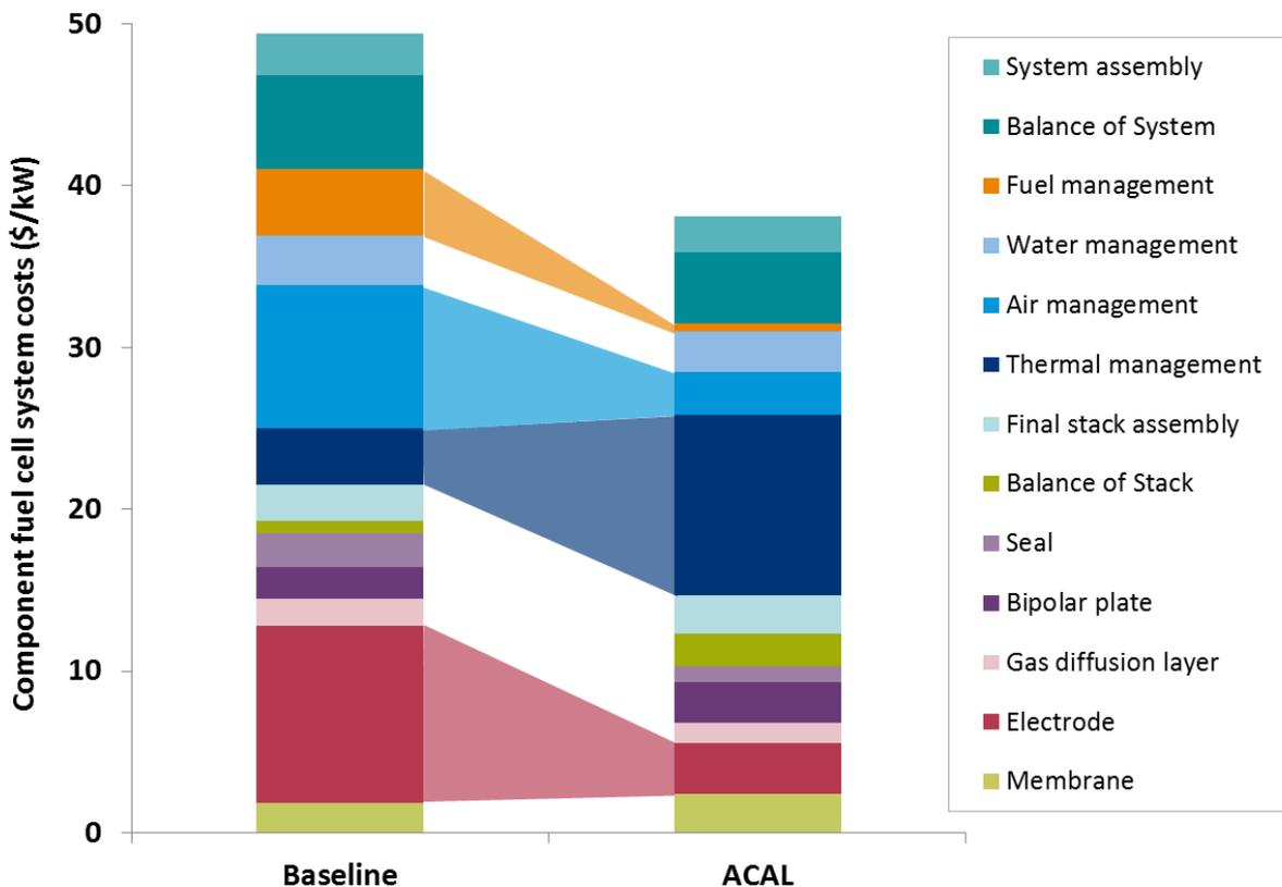
**Figure 18: How ACAL Energy's fuel cell design reduces cost compared to current industry-leading technology. The increase in thermal management costs is due to ACAL's catholyte regenerator**
