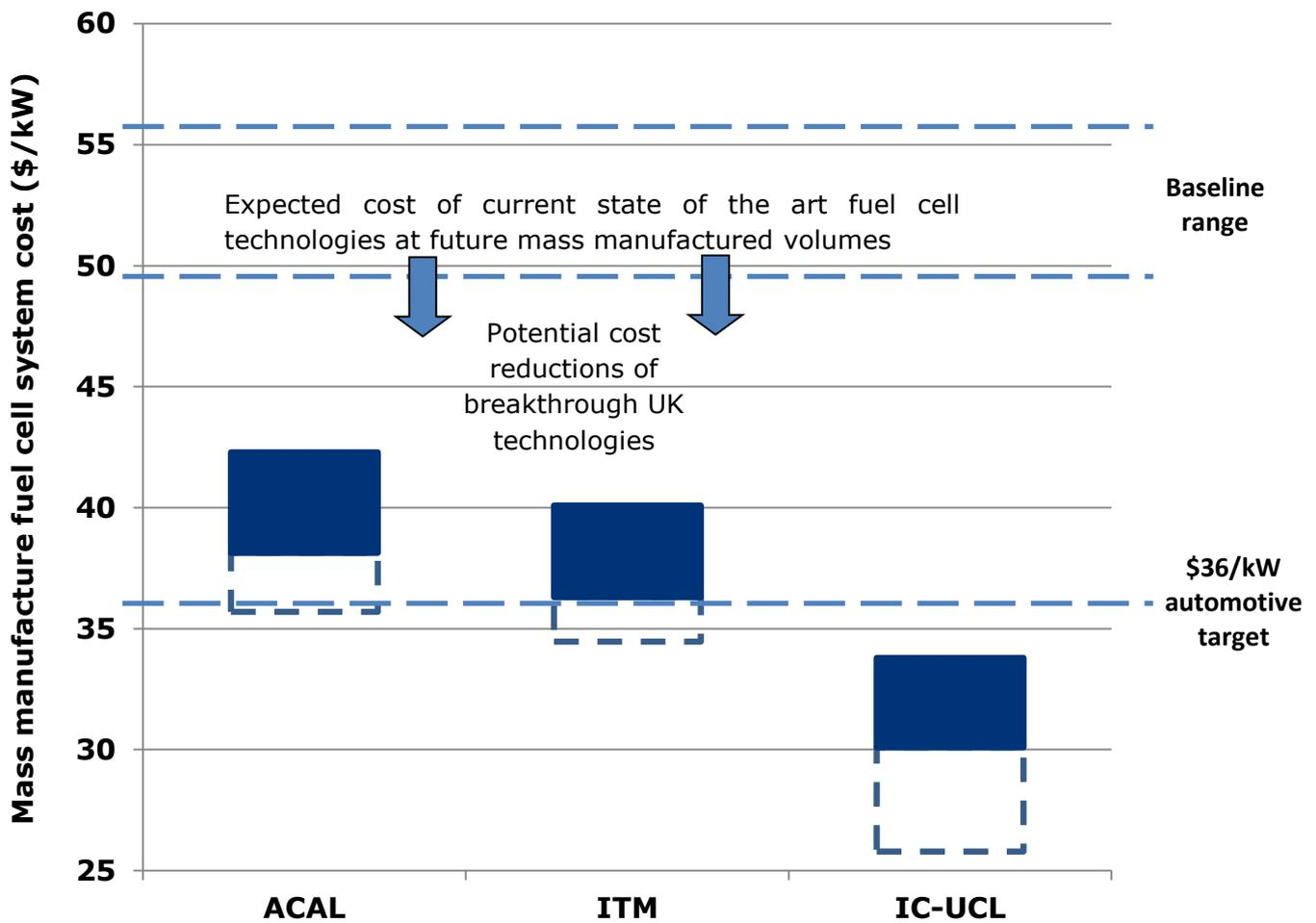
**Figure 1: Ranges of automotive fuel cell system costs at mass manufactured volume.**
