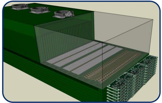
**Figure 6: Model of a Flexi-Planar stack, with cut-away**
