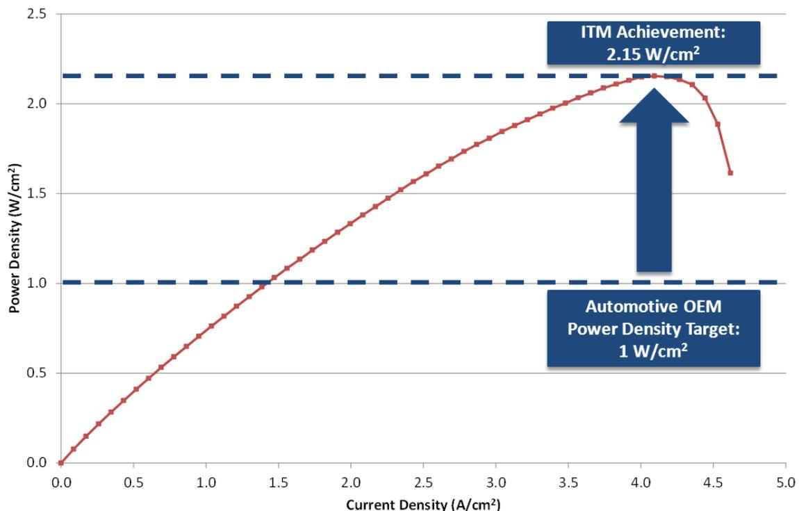
Figure 5: Performance of ITM Power membrane in  $\text{H}_2$ /air compared to automotive target
