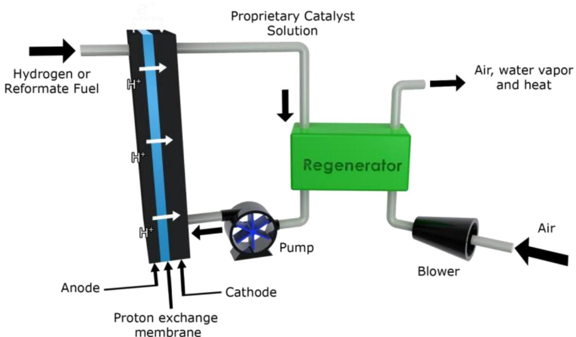
Figure 4: FlowCath® half-cell and regeneration system
