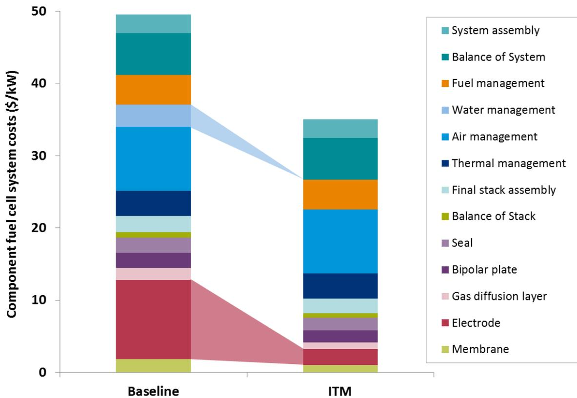
**Figure 19: How ITM Power’s fuel cell technology reduces cost compared to current industry-leading technology**
